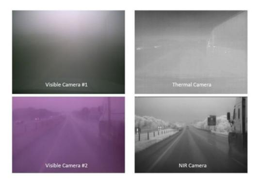
The NIR system from Bright Way Vision yielded performance unlike anything we have experienced thus far. The visible cameras (#1, #2) represented human eyes while the NIR camera could see through the dense rain. The thermal camera works well in this environment too but heat signatures are less detectable in these conditions.
