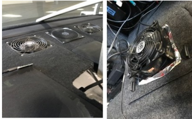
Passive thermal management solution in the trunk
