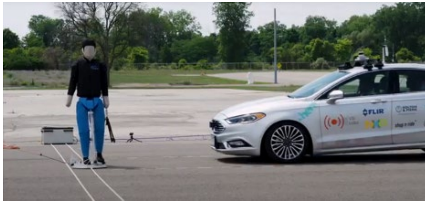
VSI Labs AEB-P Testing at ACM (Source: Teledyne FLIR)
